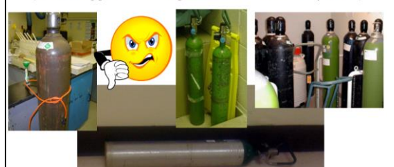
The wrong way to store gas/oxygen cylinders
